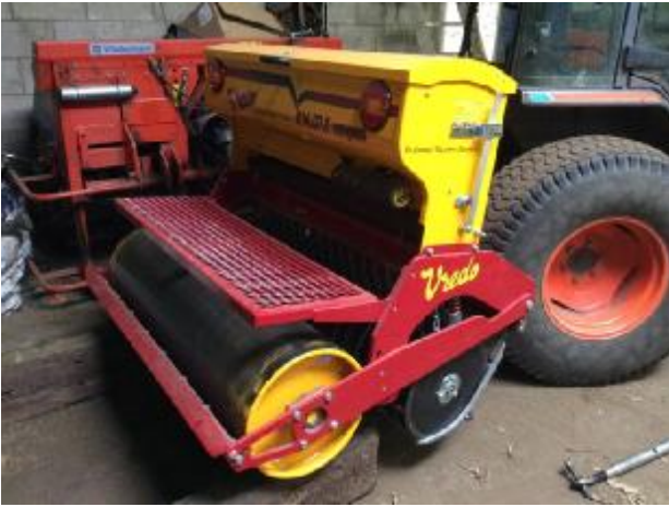
Figure 13: The acquisition of a dedicated tractor-mounted slit-seeder (Vredo) has proved an invaluable addition to the fleet at Retford GC, and in particular in the recovery of the fairways.
