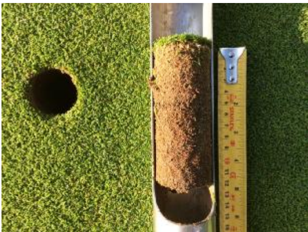
Figure 3: Inspection of the soil profile on the greens revealed a good sand integration which will aid the degradation of thatch and improve overall drainage characteristics.
